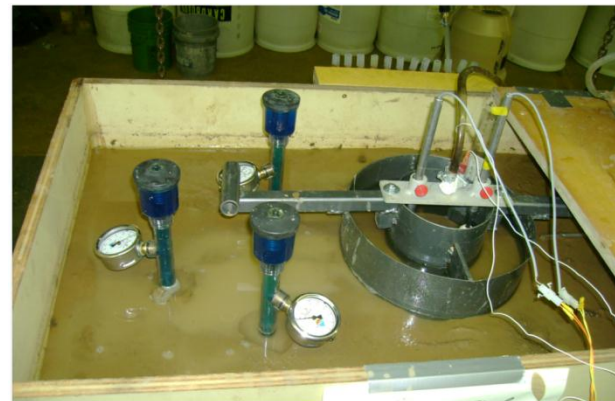
Double Ring Infiltrimeters Hydraulic conductivity
